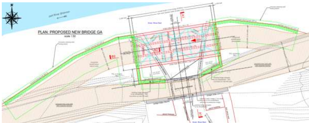
Figure 6-90: Plan for the proposed new bridge 2 alongside the existing stone bridge (refer to drawing RHA-XX-DR-S-SP0021)
